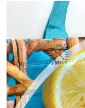
Closure with ultrasonic welding process
